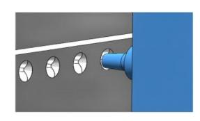
4: release the handlebar and lock in the feeder bank
